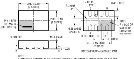
1. DRAWING CONFORMS TO VERSION (WECD-1) IN JEDEC PACKAGE OUTLINE M0-229
