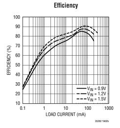
Dual 1 Cell to 1.8V, 3V Sequenced Supply
