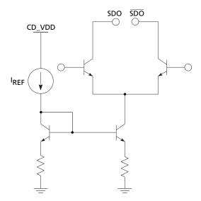
Figure 3-1: Differential Output Stage (SDO/SDO)
