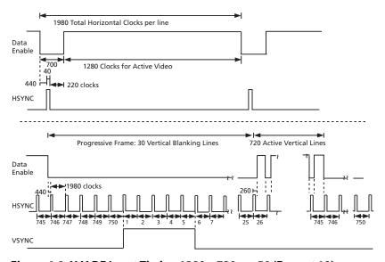
Figure 4-9: H:V:DE Input Timing 1280 x 720p @ 50 (Format 19)
