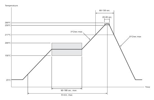
Figure 7-3: Pb-free Solder Reflow Profile
