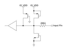
Figure 3-5: Digital Input Pin with weak pull-up maximum pull-up current <110μA (ACLK1, ACLK2,
