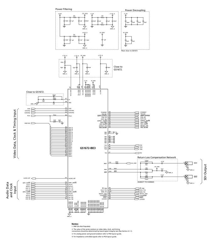
**Figure 5-1: Typical Application Circuit**
