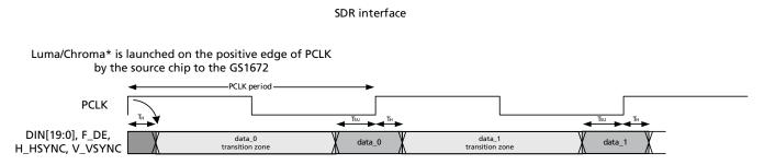
Figure 4-1: GS1672 Video Host Interface Timing Diagrams
