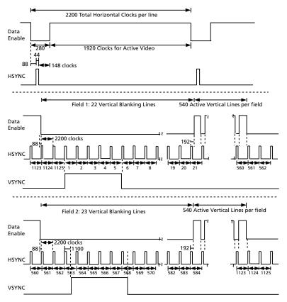
Figure 4-7: H:V:DE Input Timing 1920 x 1080i @ 59.94/60 (Format 5)
