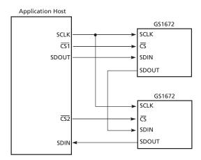
Figure 4-24: GSPI Application Interface Connection
