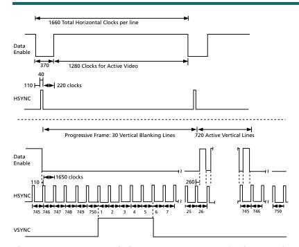
Figure 4-6: H:V:DE Input Timing 1280 x 720p @ 59.94/60 (Format 4)
