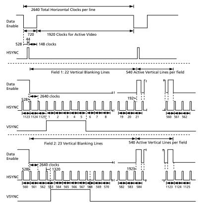
Figure 4-10: H:V:DE Input Timing 1920 x 1080i @ 50 (Format 20)
