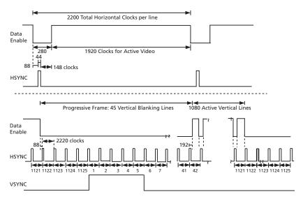
Figure 4-14: H:V:DE Input Timing 1920 x 1080p @ 29.97/30 (Format 34)
