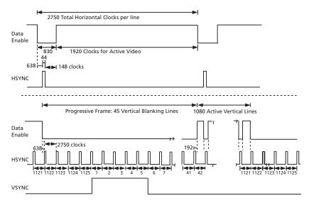
Figure 4-12: H:V:DE Input Timing 1920 x 1080p @ 23.94/24 (Format 32)
