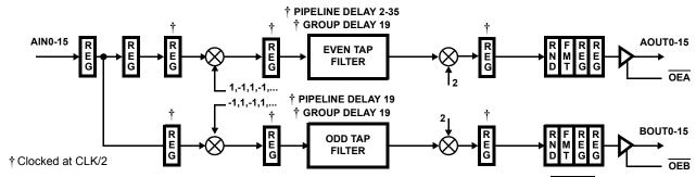
FIGURE 15A. DATA FLOW DIAGRAM FOR DOWN CONVERT AND DECIMATE MODE (INT/EXT = 1)
