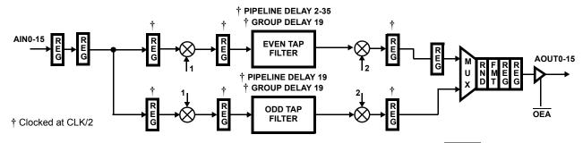
FIGURE 11A. DATA FLOW DIAGRAM FOR INTERPOLATE BY 2 FILTER MODE (INT/EXT = 1)
