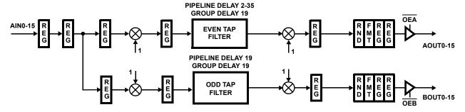
FIGURE 11B. DATA FLOW DIAGRAM FOR INTERPOLATE BY 2 FILTER MODE (INT/EXT = 0)
