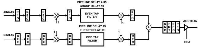
FIGURE 7B. DATA FLOW DIAGRAM FOR DECIMATE BY 2 FILTER MODE (INT/EXT = 0)
