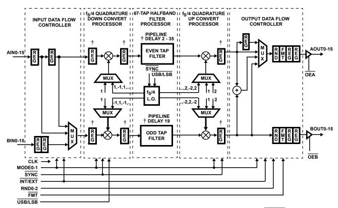
† Indicates elements which operate at CLK/2 when the INT/EXT control input is high.
