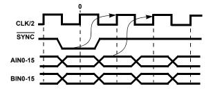
FIGURE 22. DATA <u>SYNCHR</u>ONIZATION WITH PROCESSING LEGS (INT/EXT = 1)
