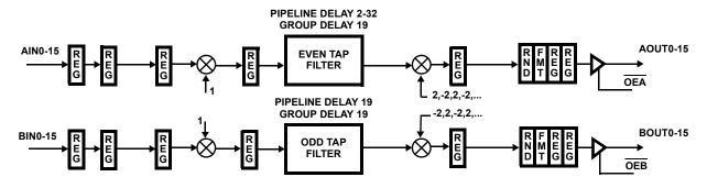
FIGURE 21B. DATA FLOW DIAGRAM FOR QUADRATURE TO REAL CONVERSION MODE (INT/EXT = 0)
