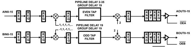
FIGURE 15B. DATA FLOW DIAGRAM FOR DOWN CONVERT AND DECIMATE MODE (INT/EXT = 0)
