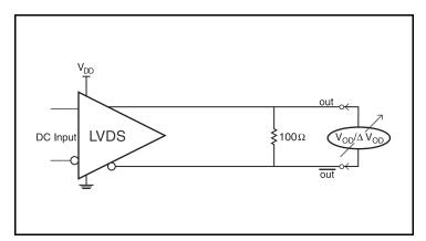
**Differential Output Voltage Setup**
