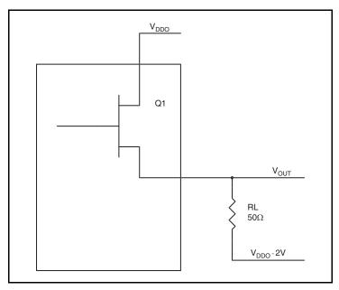
Figure 8. LVPECL Driver Circuit and Termination
