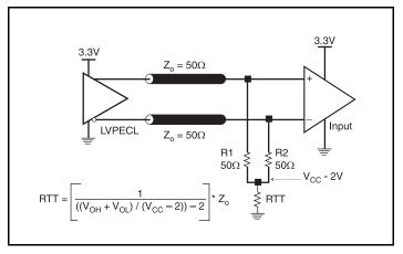
Figure 4A. 3.3V LVPECL Output Termination
