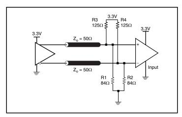
Figure 4B. 3.3V LVPECL Output Termination
