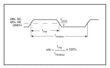
**Differential Output Duty Cycle/Pulse Width/Period**
