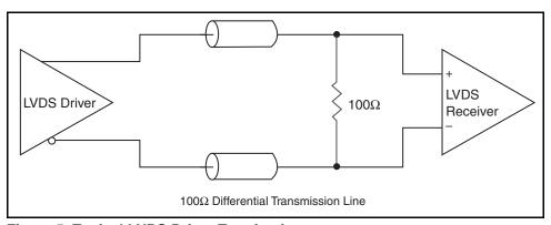
Figure 5. Typical LVDS Driver Termination
