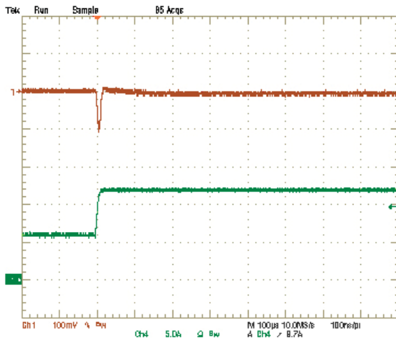
Step Load Transient Response (Vin=5.0V, Vout=2.5V, Cload=94µF, Iout=6A to 12A) Trace 1=Vout, 100 mV/div, Trace 4=Iout, 5A/div.
