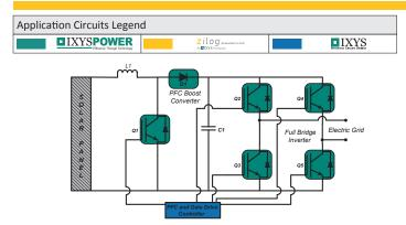
Figure 1: Solar Inverter
