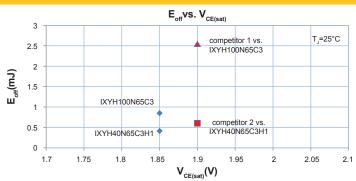
These 650V XPT $^{\text{TM}}$  IGBTs are designed to achieve an optimal balance between the turn-off energy loss and on-stage voltage, especially in hard-switching applications. The graph demonstrates a superior trade-off of the new IGBTs (in particular, the IXYH100N65C3 against competitor 1 and IXYH40N65C3H1 against competitor 2).
