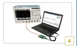
• Connect J7 and J8 using SMA cables to an Oscilloscope to evaluate the pre-programmed 114.285 MHz LVDS Clock
